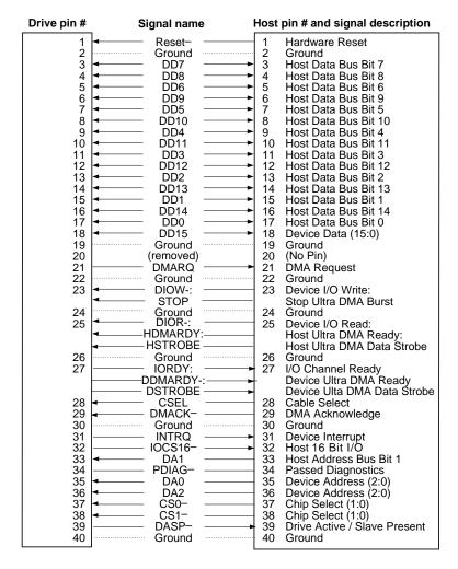
Pins 28, 34 and 39 are used for master-slave communication (details shown below).
