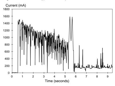
Figure 1. Typical startup and operation current profile for the ST34342A and ST33232A
