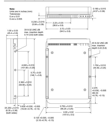
Figure 4. Mounting dimensions—top, side and end view
