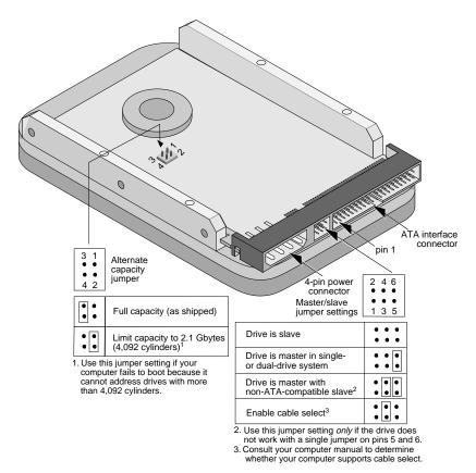
Figure 3. Alternate capacity jumper (ST34342A and ST33232A only) and master/slave jumpers
